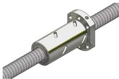
Figure 1.13 __ Single flange type nut with pitch offset
